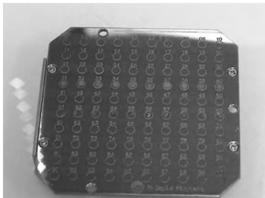
Fig. 10.16. Photograph of a MALDI sample plate able to take 100 deposits. A few crystal samples are visible
