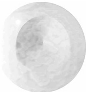
Fig. 25.12. Scanning electron microscope (SEM) image of Trisacryl spheres
