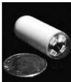
Fig. 26.1. M2A minicapsule. Length 30 mm, diameter 11 mm
