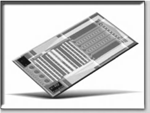
Fig. 26.3. Lab-on-a-chip. PCR amplification and detection of DNA [5]
